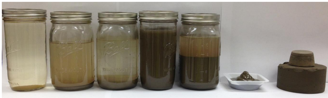
Figure 4. Progression of FGD purge water in the Heartland Concentrator from raw feed to solidified and stabilized residual.
